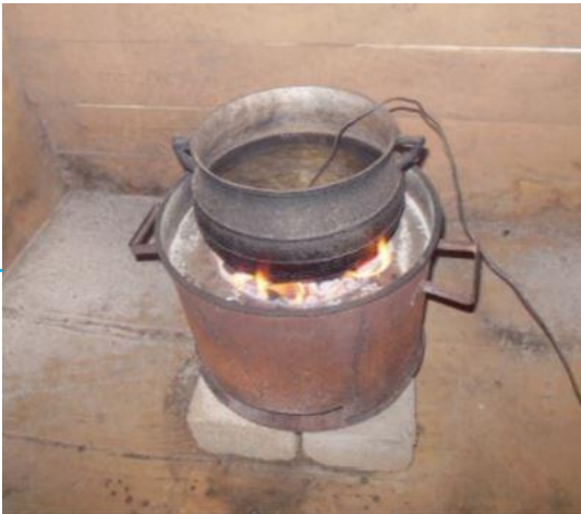
Fig. 7. Briquette combustion in the Water Boiling Test.
