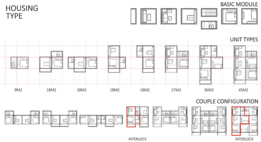
Fig. 12 Housing type modular system. (Source Author)
