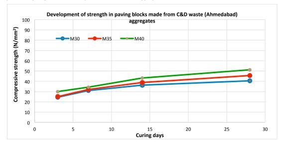
M30 grade paving block achieved 100% strength within 7 days while in M35 and M40 grade strength was achieved within 14 days. The rate of strength increase is similar in M30 and M35 grades of paving block but M40 grade paving block has an improved strength development. On an
