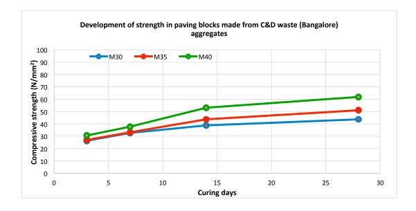
All grades of paving block achieved designated strength within 7 days. The rate of strength increase was similar in M30 and M35 grades of paving block. M40 paving block has a distinct strength build up pattern. An average of 45% higher strength was seen in all grades for paving block using Bengaluru C&D waste (compared to standard for paving blocks made with natural aggregates).
