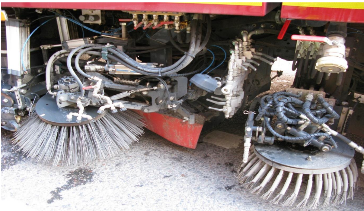
Figure 9. Brushes and spraying equipment on a cleaning machine. Photo: Mats Gustafsson, VTI
