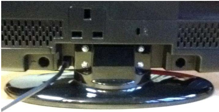
Figure 59 Poor attachment of the stand of a TV set with screws
