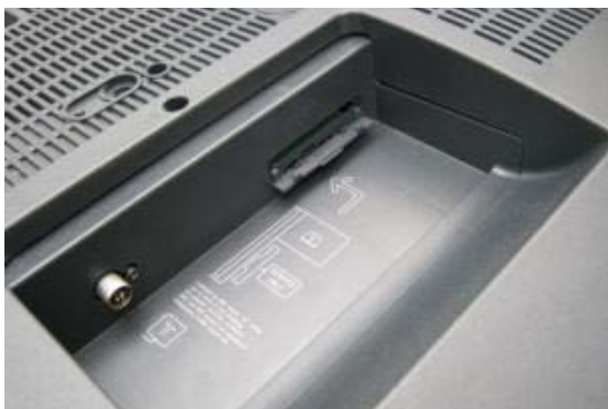
Figure 64 Interface for reading out information for repairs or for updating the software
