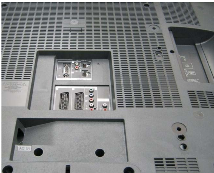
Figure 58 Recessed positioning of ports and sockets to protect them against mechanical impacts
