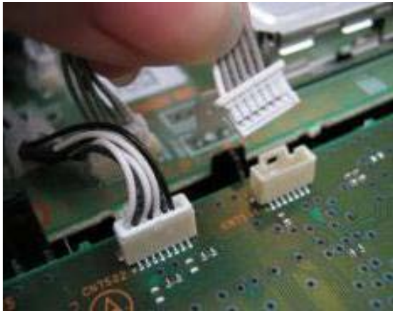
Figure 61 Plug-in connections between circuit boards
