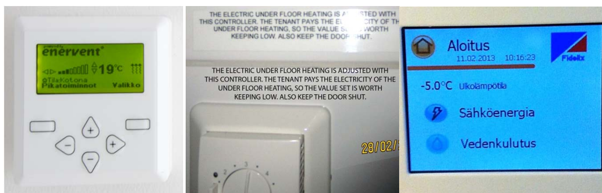
Figure 19: Tenants may adjust ventilation settings, control underfloor heating, and follow their electricity and water use. Radiators can be adjusted. The use of the cooker extractor fan automatically reduces the ventilation unit fan power, to balance the apartment air pressure.
