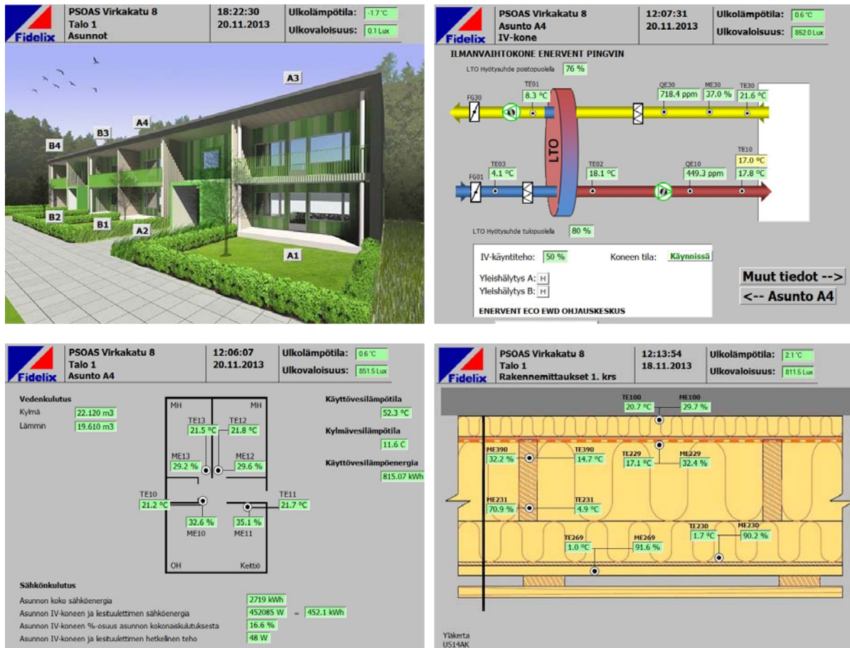
Figure 16: Screenshots from the online interface of the digital building automation system accessing monitoring data. Top left image shows the links to the monitoring data from eight apartments A1-B4. Top right image displays monitoring parameters as collected from all eight apartment ventilation units. Bottom-left image displays household energy use, and indoor temperature and relative humidity data as monitored in two apartments. Bottom right image displays building physics monitoring of temperature and relative humidity in one of the four monitored façade locations (Palosaari M, Fidelix. 2013)
